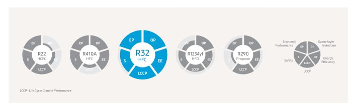
The EHS Mono and Split range uses the next generation of R32 refrigerant, which helps and lower the impact on global warming. It is equipped with an Ozone Depletion Potential (ODP) of zero and a lower Global Warming Potential (GWP) than conventional R22 or R410A refrigerants1. It also reduces the amount of refrigerant needed and cuts CO<sub>2</sub> emissions<sup>2</sup>, so it's much more environmentally friendly.
